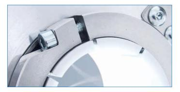
sleeve and the shaft as well as an integrated lock nut prevent them from accidentally falling out. Nevertheless it is possible to dismantle the insulating sleeve and replace it in order to fit a different shaft diameter.
